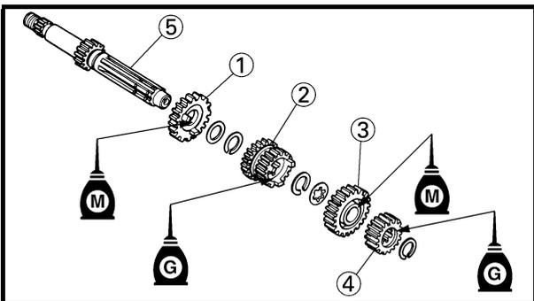
**INSTALLING THE TRANSMISSION**
