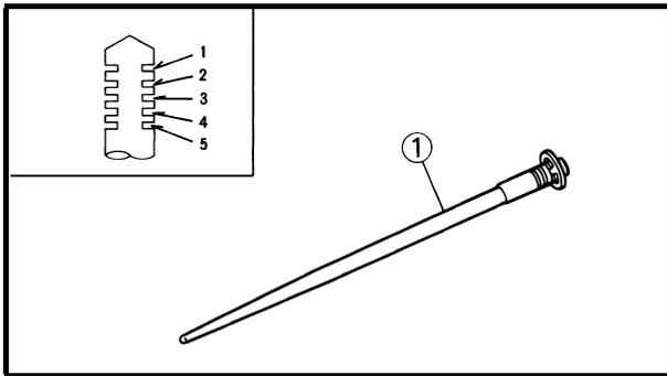
**JET NEEDLE GROOVE POSITION ADJUSTMENT**
