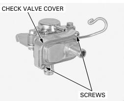
Check the reed for damage or fatigue, replace the PAIR control valve if necessary. Replace the PAIR control valve if the check valve rubber seat is cracked, deteriorated, damaged or if there is clearance between the reed and seat.
