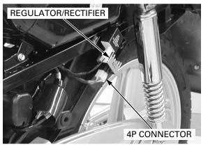
If all components of the charging system are normal and there are no loose connections at the regulator/ rectifier connectors, replace the regulator/rectifier unit (page 15-11).
