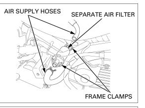
Check the separate air filter, replace it if necessary.This separate air fil-Installation is in the reverse order of removal.
