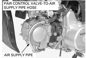
Check the air supply hoses for damage or loose connections.
