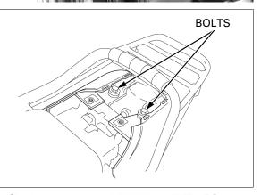
Remove the two brake/tail light mounting bolts.
