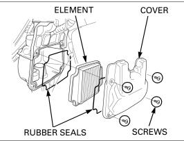
Clean the air cleaner element using compressed air from the carburetor side, or replace it according to the maintenance schedule (page 24-23).
