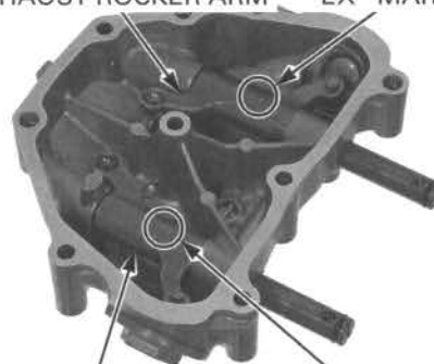
INTAKE ROCKER ARM "IN" MARK
