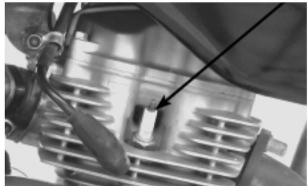
**REEMPLAZO DE LA BUJIA DE ENCENDIDO**
