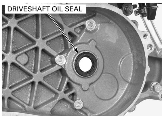
Apply engine oil to the bearing cavity.
