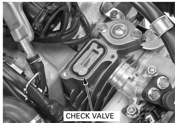
Check the reed for damage or fatigue. Replace if necessary.
