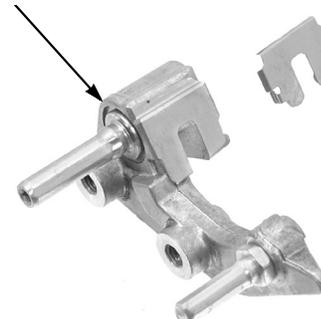
Remove the pin boots and pad spring from the brake caliper.
