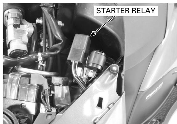
**STARTER RELAY COIL LINE INSPECTION**
