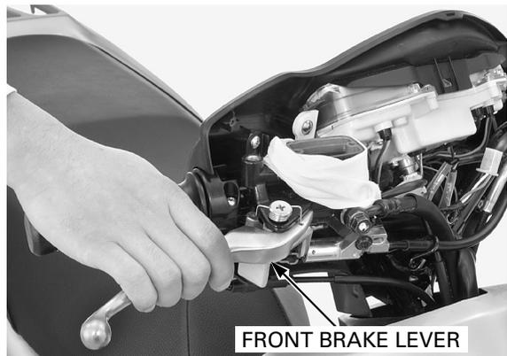
*Do not release the brake lever until the bleed valve has been closed.*
