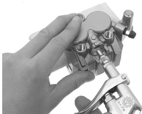
*Be careful not to damage the piston sliding surface.*
