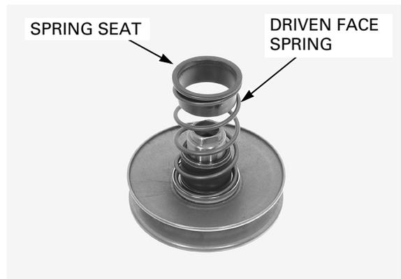
Set the clutch assembly to the driven pulley.
