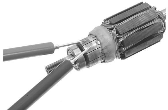
Check for continuity between each commutator bar and the armature shaft.
