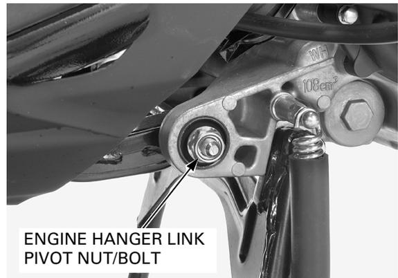
Remove the engine hanger link pivot nut (frame side).
