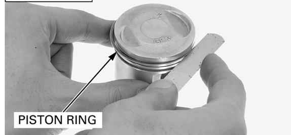
Insert each piston ring into the bottom of the cylinder squarely using the piston. Measure the ring end gap.
