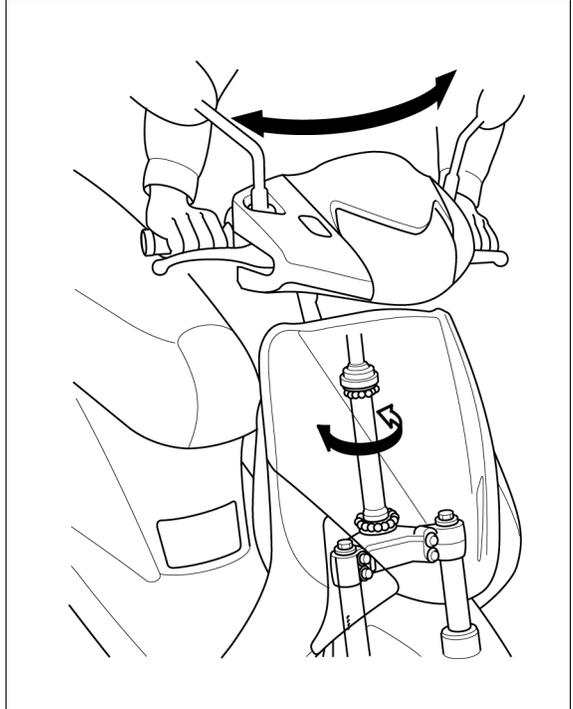
Hold the scooter and check the steering head bearings for wear by moving the fork forward and backward.
