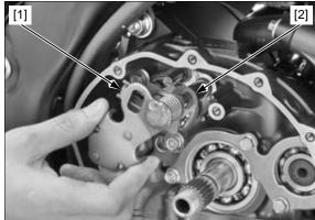
Remove the shift drum center socket bolt [1].
