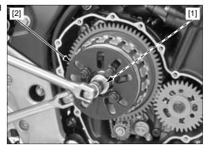
Remove the lock washer [1] and washer [2].
