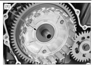
Align the primary drive (scissors) gear teeth by inserting a screwdriver into the gear slot [1] and prying the gears, and install a 6 x 14 mm bolt [2] into the primary drive gear holes.
