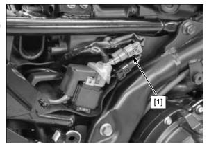
Check for continuity between each terminal of the sensor side rear wheel speed sensor 2P (Gray) connector [1] and ground.
