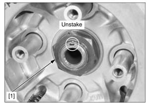
Hold the clutch pressure plate with the special tool and loosen the clutch center lock nut [1].
