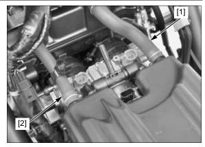
throttle cables [1] (remove from the cable holder and disconnect from the throttle drum)
