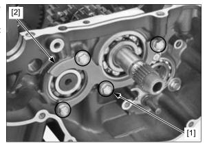
Position the balancer shaft with the left balancer weight [1] facing up.
