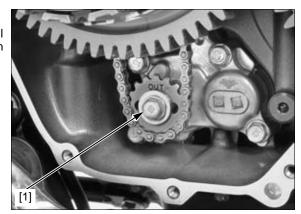
Remove the clutch lifter rod B [1].
