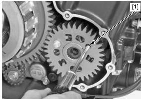
Apply engine oil to the primary drive gear bolt threads and seating surface.
