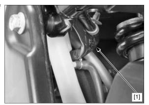
Remove the bolt [1] and clutch cable holder [2], then disconnect the clutch cable [3] from the clutch lifter arm [4].
