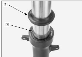
Using quick successive motions, pull the fork tube out of the fork slider.
