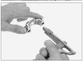
Apply molybdenum oil solution to the crankpin bearing sliding surfaces on the crankpin bearing caps.
