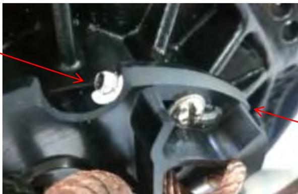
**Pic. 2.1.** Unscrew 2 lateral allen screws.
