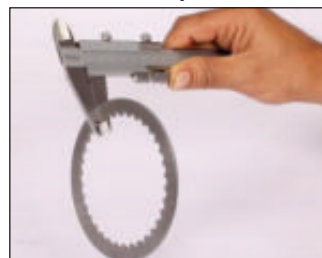
Steel Plate Warp
