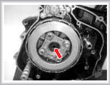
Clutch Nut (LH Threads)
