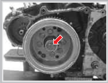
Rotor Mounting Bolt
