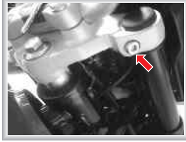
Upper Clamp Allen Bolt
