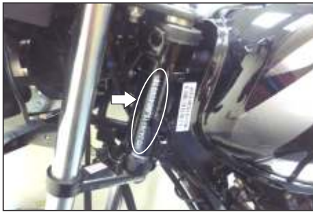
▶ Frame Number Location On Side of Steering Tube (Alpha-Numeric - 17 Digits)
