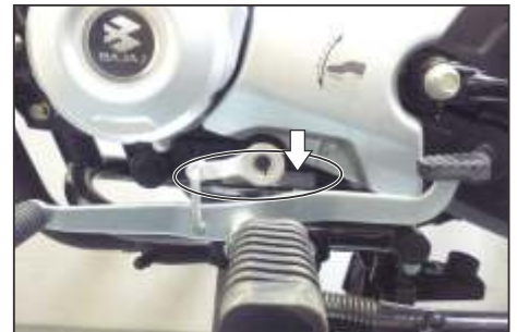
◀ Engine Number Location On LH Side Crankcase Near Gear Change Lever (Alpha-Numeric - 11 Digits)
