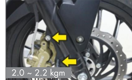
Front Caliper Mounting Bolt
