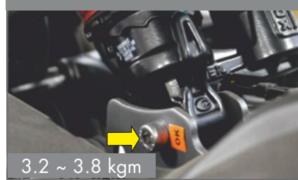
Front Caliper Mounting Bolt
