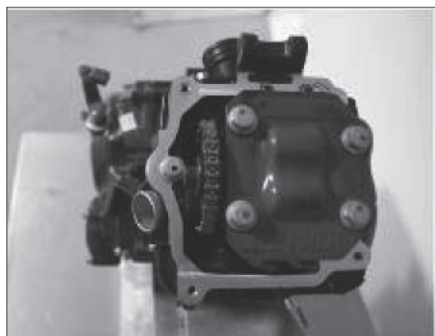
Cylinder Head Bolts (12 mm)
