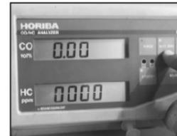
Carry out Span Check as per manufacturer's Recommendation to confirm the OK condition of the Equipment (If Span Check does not confirm the reading, then carry out Gas Calibration as per mfgs. recommendation). Set the Equipment display to Zero before taking the reading.
